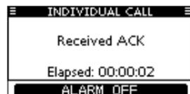
Push [ALARM OFF] to stop the beeps, and then select the intership channel specified in step ④.
