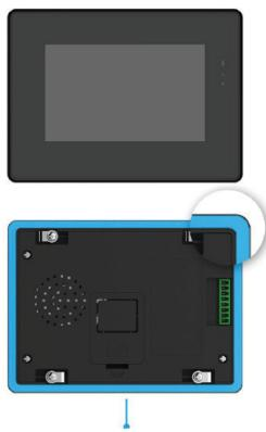
Waterproof rubber gasket (blue part in the schematic, actually in black): located between screen and shell to prevent water ingress. Additional glass glue is available for outdoor use to strengthen the waterproof performance
