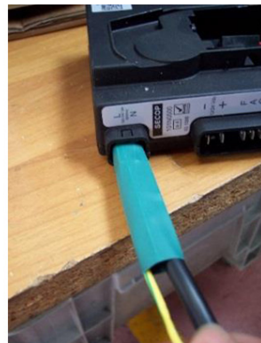
Figure 11: Detail of double insulated connection
